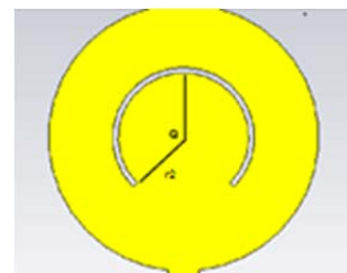
Figure 12: Antenna structure for 3.5 GHz notch
