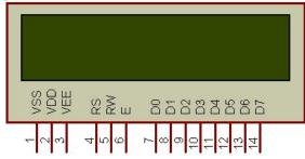
In this tutorial, we will discuss about character based LCDs, their interfacing with various microcontrollers, various interfaces (8-bit/4-bit), programming, special stuff and tricks you can do with these simple looking LCDs which can give a new look to your application Most LCDs with 1 controller has 14 Pins and LCDs with 2 controller has 16 Pins (two pins are extra in both for back-light LED connections).
